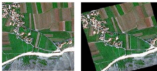
Fig.3. « l'île de Ré » High Resolution (HR) multispectral satellite images pair. SPOT 5 (2.5m) image before (left) and after rigid transformation (right)
